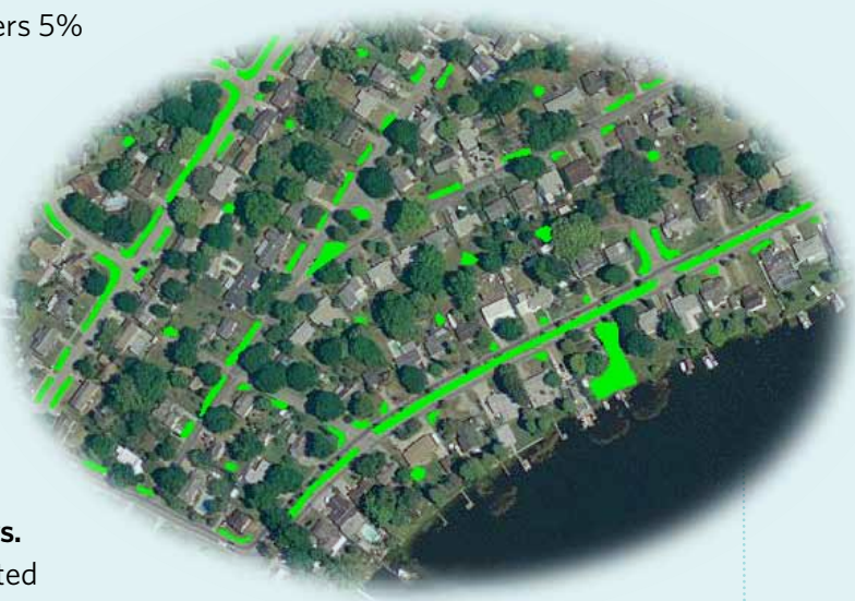
FIGURE 14. Aerial photo of a residential neighborhood in southwest Winter Haven, showing a stormwater capture system that covers 5% of the surface area (highlighted in green).
